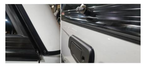
6. Measure and record the gap between the tub rail and the inside lip of the canopy base rail on each side of the vehicle – these measurements should be similar on each side. Record the measurement.
