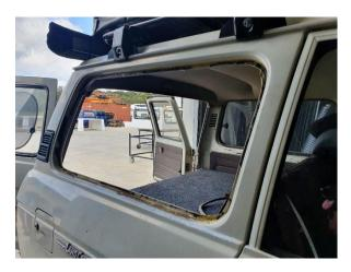
2. PUSH ON THE PINCHWELD ON TO THE EXPOSED EDGE WITH THE BUBBLE SEAL FACING OUTWARDS.
