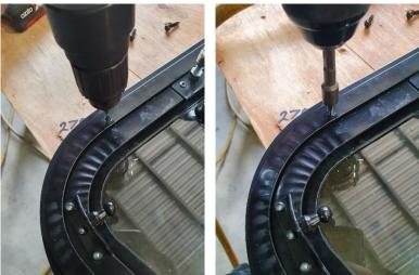
4. REMOVE THE Z ALLOY AND PLACE THE WINDOW IN TO THE HOLE. ENSURE THE BUBBLE SEAL HAS TAKEN UP ANY GAPS IN THE CORNERS.
