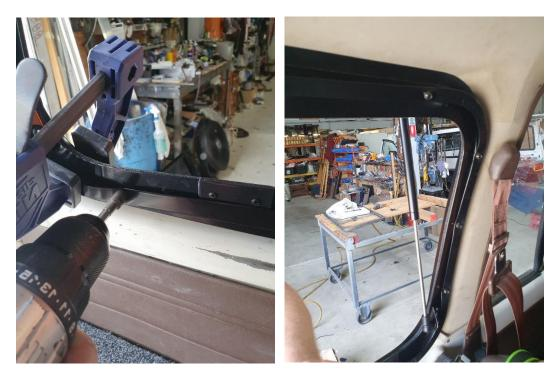
IF THE WINDOW GETS HARD TO OPEN OVER TIME – ADJUST THE BOLT ON THE BACK OF THE LOCK TO ADD MORE PRESSURE ONTO THE OUTSIDE FRAME.
