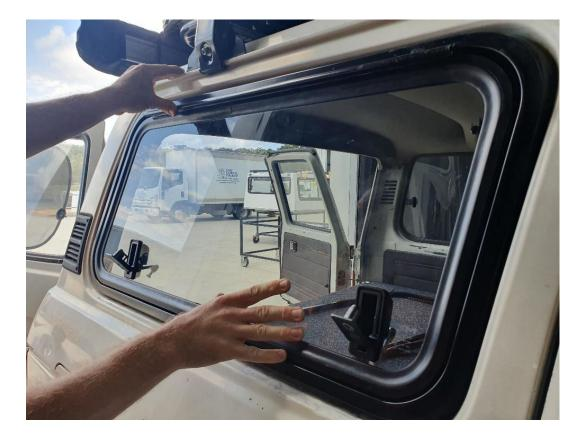
5. OPEN THE WINDOW. PLACE THE Z FRAME ON THE BACK OF THE WINDOW INSIDE THE CAR, THEN USING A G CLAMP, SQUEZE THE FRAME AND WINDOW TOGETHER NEXT TO ONE OF THE SCREW HOLES. ONCE IN PLACE, SCREW THROUGH THE HOLE INTO THE WINDOW SO IT IS JUST OVER FINGER TIGHT. COMPLETE THIS PROCESS ON ALL SCREW HOLES, THEN CHECK THE RUBBER ON THE OUTSIDE IS COVERING ALL GAPS AND THE WINDOW APPEARS TO BE SITTING SQUARE. THEN TIGHTEN ALL SCREWS UP INSIDE.
